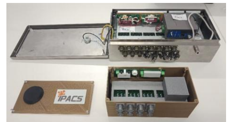
Compact and easily transportable: 3D printed proto-type model of a new Data Acquisition System
